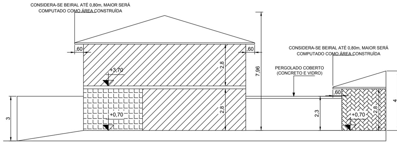
CORTE A - A (ESQUEMÁTICO)
